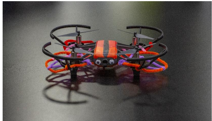
Figure 1: The drone Walden is shaped like a butterfly, because users naturally know how to interact with concepts that are familiar to them.
